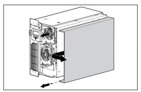
Figure 2-7. Removing the U-channel access panel
